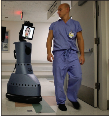
The Remote Presence Robot (RP-7) from InTouch Health is a mobile telemedicine unit that connects physicians and specialists with patients and other doctors in real time through computers equipped with cameras and microphones.
