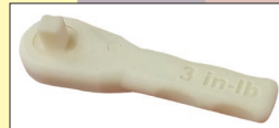
THIS RATCHET WRENCH WAS MADE USING A 3-D PRINTER ON THE INTERNATIONAL SPACE STATION IN ABOUT FOUR HOURS. © NASA/Spa USA/ Newscom
